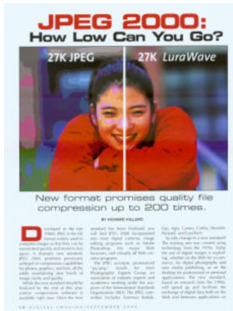
Figure 3: Scanned document compressed with LuraDocument. 7,204 KB original TIFF file compressed down to 37 KB as a LuraDocument.
